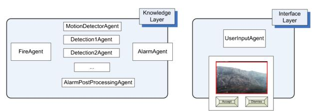
Fig. 13. Fire detection holon. (Colors are visible in the online version of the article; http://dx.doi.org/10.3233/AIC-130567.)
