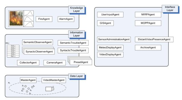
Fig. 7. Multi agent observer network shell. (Colors are visible in the online version of the article; http://dx.doi.org/10.3233/AIC-130567.)
