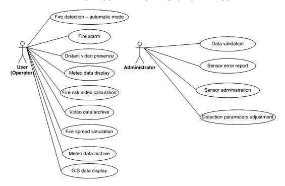
Fig. 2. Use case diagram of iForestFire system.
