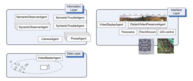
Fig. 12. Video holon. (Colors are visible in the online version of the article; http://dx.doi.org/10.3233/AIC-130567.)
