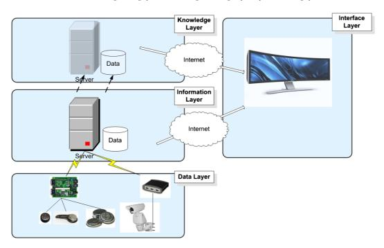
Fig. 15. Hardware elements of iForestFire. (Colors are visible in the online version of the article; http://dx.doi.org/10.3233/AIC-130567.)
